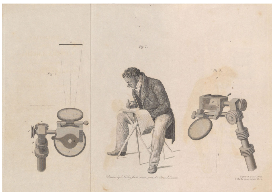
An illustration of the camera lucida, from George Dollond's Description of the Camera Lucida: An Instrument for Drawing in True Perspective, and for Copying, Reducing, or Enlarging Other Drawings (1830).
